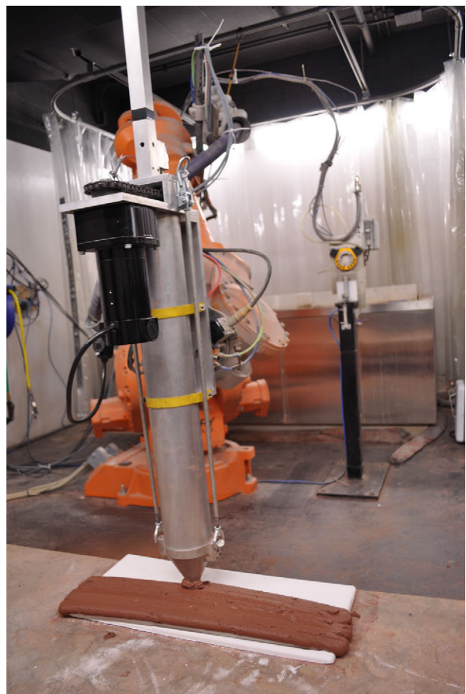
Figure 2. 3D printing test over a plaster mold.
