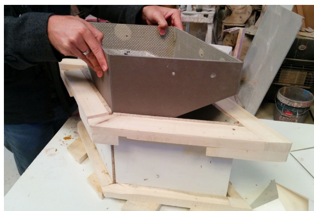
Figure 12. Female molds were used to assembly precise modules that, once stacked and bolted together, formed a structurally active prototype (Photo: Jordi Font de Mora, Grupo on Market).
