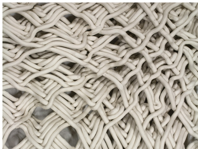
Figure 8. 3D printed ceramic pattern. Study by Jared Friedman, Olga Mesa, and Hea Min Kim at Harvard GSD. Instructors: Nathan King, Rachel Vroman (Photo: Jared Friedman).
