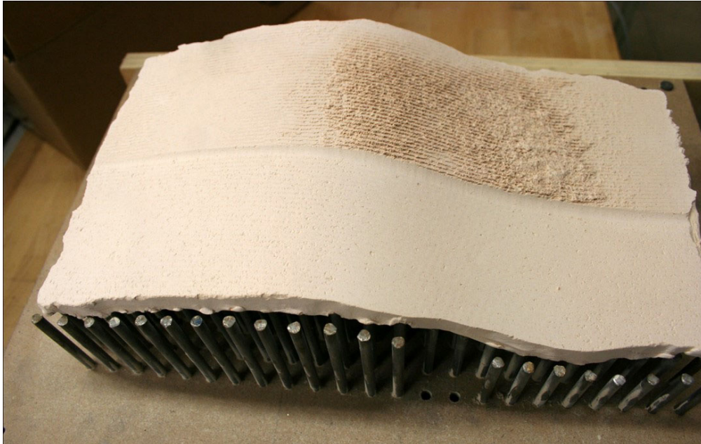
Figure 5. Clay prototype produced over an actuated pin mold. Surface quality was improved through robotic milling as post-processing operation.
