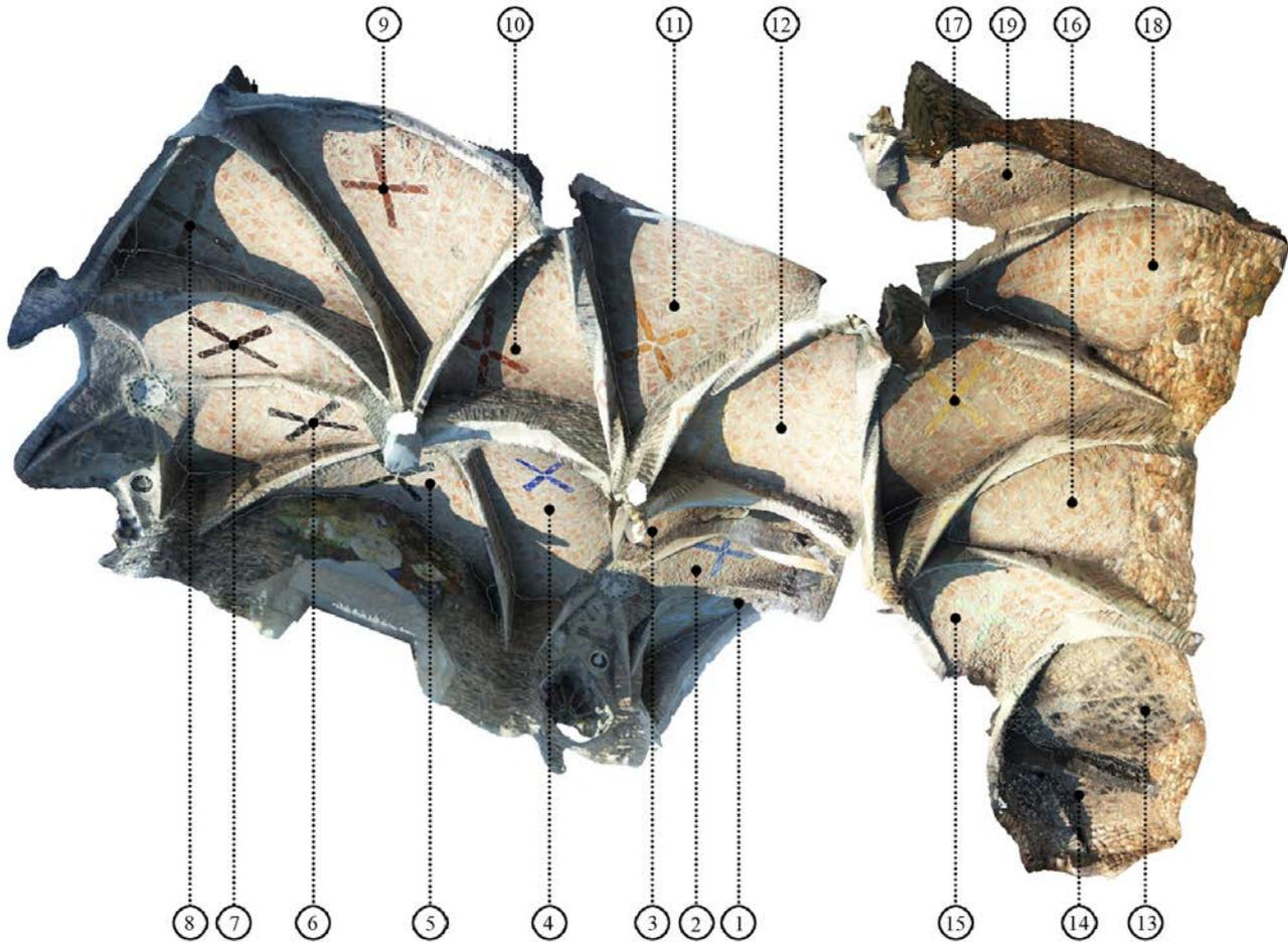
Figure 2. Three-dimensional model of the 19 vaults forming the entrance porch to the crypt. [Image generated by the authors].
