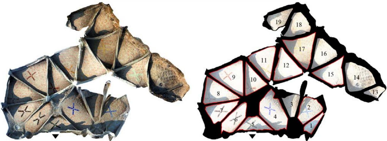
Figure 3. Orthogonal projection on the ground plane of the 19 vaults forming the entrance porch to the crypt. In the right image, the 13 vaults which bear a coloured ceramic cross on their surfaces are highlighted in red. The triangle pinpoints the location of the entrance to the crypt. [Image generated by the authors].
