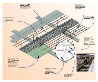
Figure 7. Example of Mobile Guardrail for Leading Edge Work (Photograph courtesy of Rossway Dowd Safety Systems Company).
