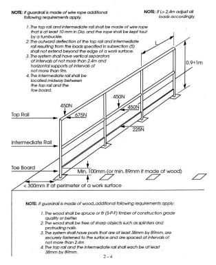
Figure 3. Guardrail According to Ontario Reg. 145-00.
