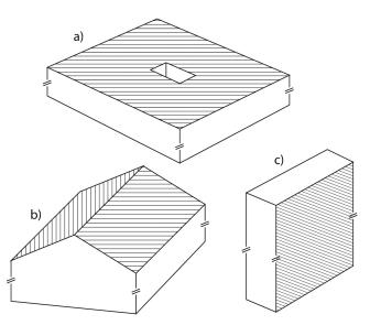
Figure 2. Fall Hazard Work Spaces Suitable for Employment of Collective Fall Protection Systems. a) Flat FHWS; b) Sloped FHWS; c) Vertical FHWS.
