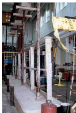
Figure 7. Wooden guardrail attached to shoring jacks with # 16 binding wire - Overlapping of guardrails on a shoring jack.
