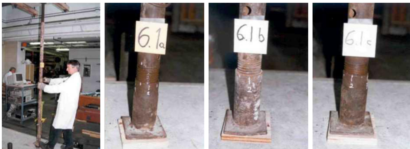
Figure 4. Tests 1-1a, 1-1b and 1-1c to determine the compressive force in a shoring jack.
