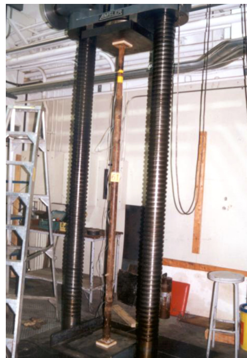
Figure 3. Calibration of a shoring jack with the Amsler press.
