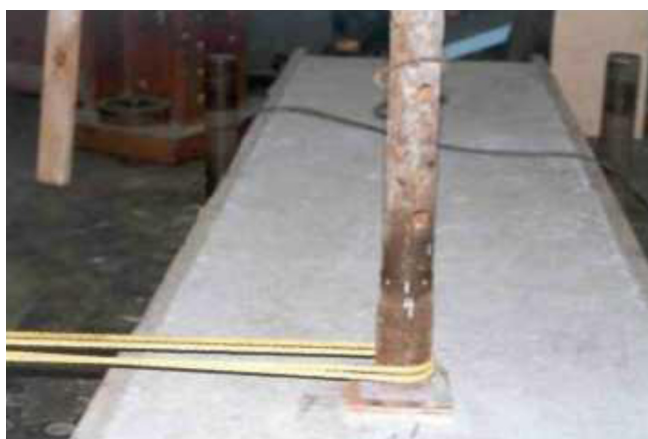
Figure 6. Determination of the friction force and the coefficient of static friction \mu .
