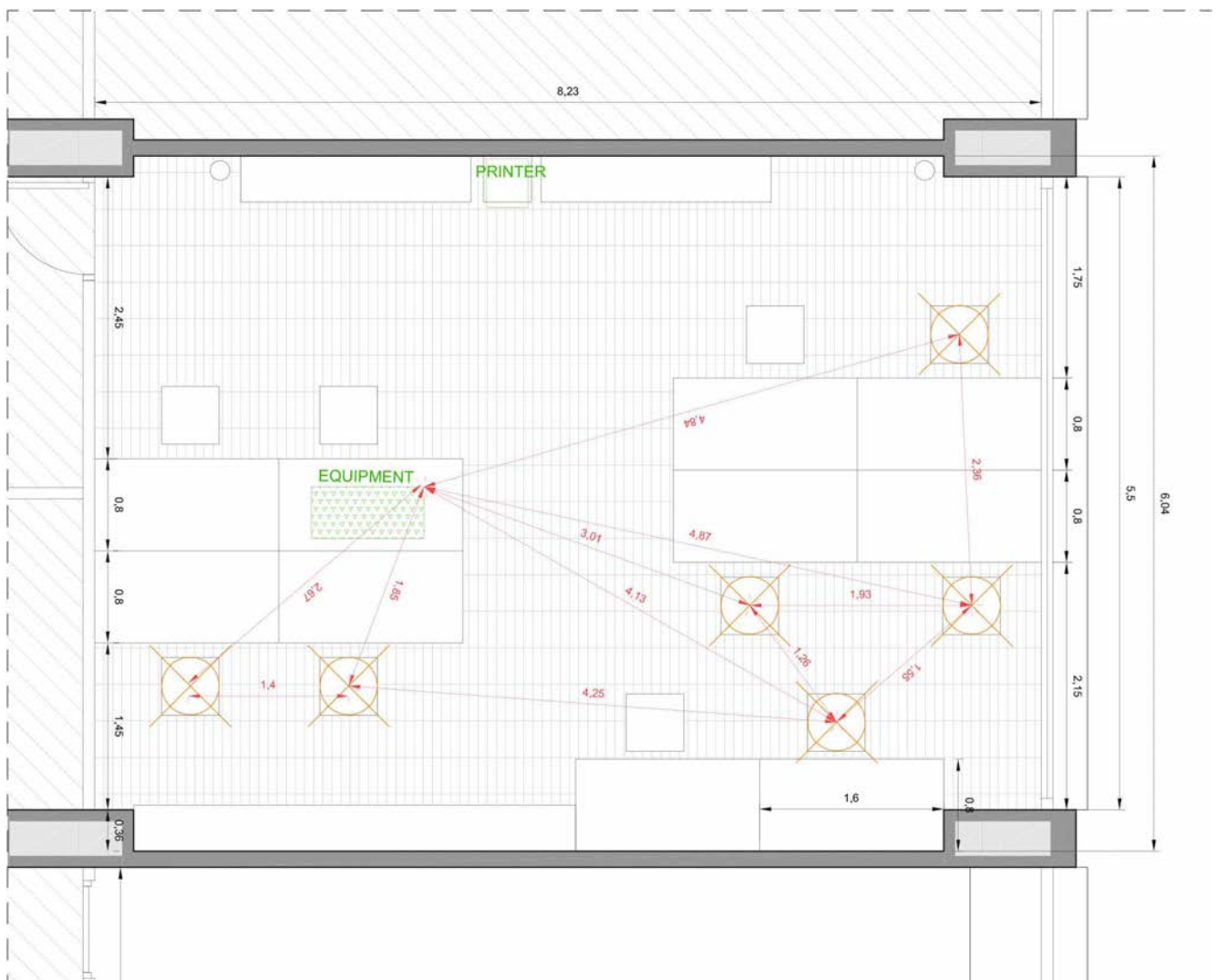
Figure 4. IEQ equipment and space distribution in an IVE open-plan office.
