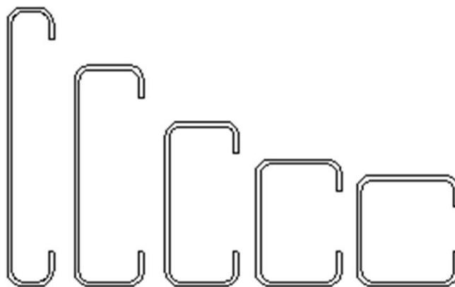
Figure 1. Possible proportions of Lipped C section with a constant developed length
