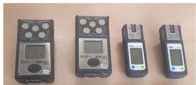
Figure 2. Real-time gas monitor device IBRID MX6 and the DRÄGER X-AM 5000.
