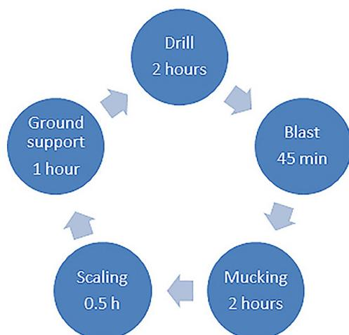
Figure 1. Simplified cycle in tunnel construction.
