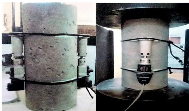
Figure 2. Modulus of elasticity test on cylinder.
