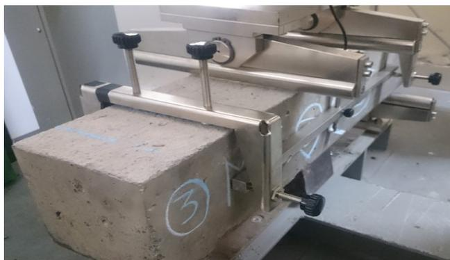
Figure 1. Flexural testing on beam.
