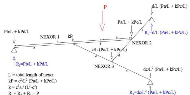
Figure 8. Basic unit of 3 nexors with  $P$  load in any position.
