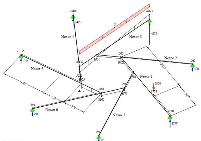
Figure 14. Shear distribution of a basic unit of 7 nexors with any point load and any uniformly distributed load (external loads [N] and [N/mm], support reactions [N], internal forces  $V_z$  [N], nexor length [mm]).
