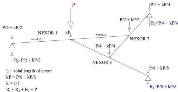
Figure 6. Basic unit of 3 nexors with  $P$  load centred on a member.
