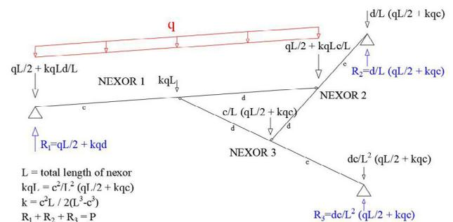
Figure 11. Basic unit of 3 nexors with uniformly distributed  $q$ -load.
