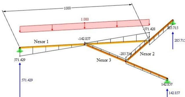
Figure 12. Shear distribution in a basic unit of 3 nexors connected by their midpoints, with uniformly distributed load on one of their members (external loads [N/mm], support reactions [N], internal forces  $V_z$  [N], nexor length [mm]).
