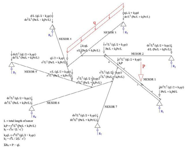
Figure 13. Basic unit consisting of 7 nexors with any point load and any uniformly distributed load.
