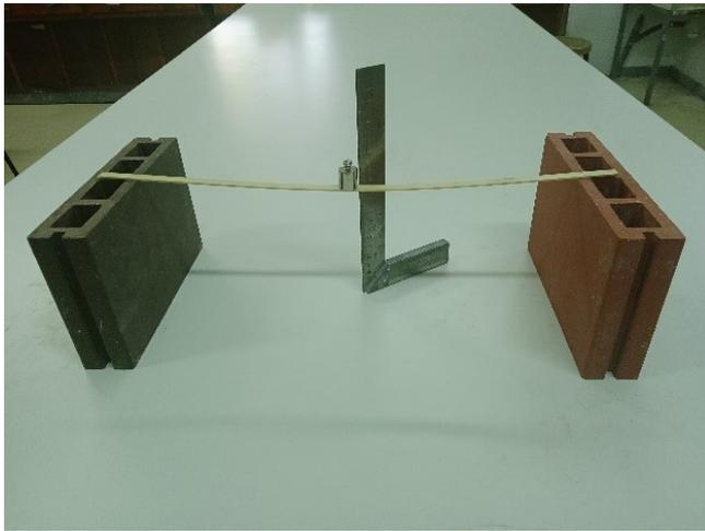
Figure 3. Vertical deflection in the centre of the span of a simple member.
