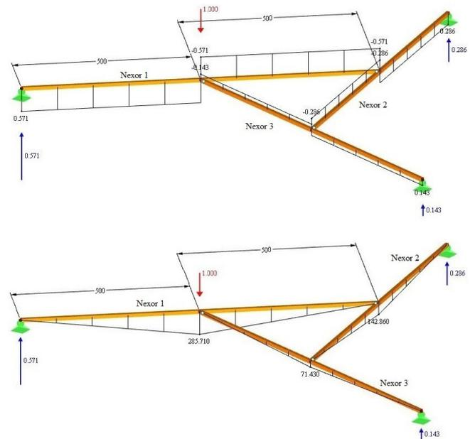
Figure 7. Shear and bending moment distribution in a basic unit of 3 nexors connected by their midpoints, with point load centred on member 1 (external loads [N], support reactions [N], internal forces  $V_z$  [N] and  $M_y$  [Nmm], nexor length [mm]).
