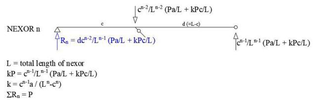
Figure 10. Load distribution on member  $n$  for a basic unit of  $n$  nexors.
