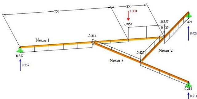
Figure 9. Shear distribution in a basic unit of 3 nexors connected by their midpoints, with point load not centred on member 1 (external loads [N], support reactions [N], internal forces  $V_z$  [N], nexor length [mm]).
