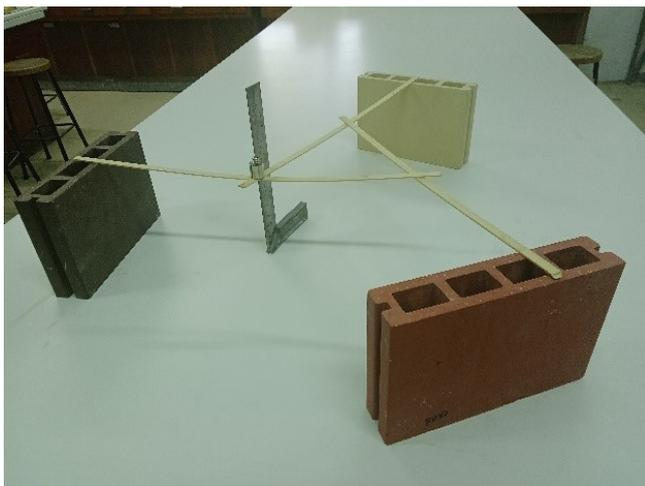
Figure 4. Vertical deflection in the centre of the span of member into reciprocal structure.
