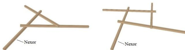
Figure 2. Basic units, or fans, of 3 nexors and 4 nexors.
