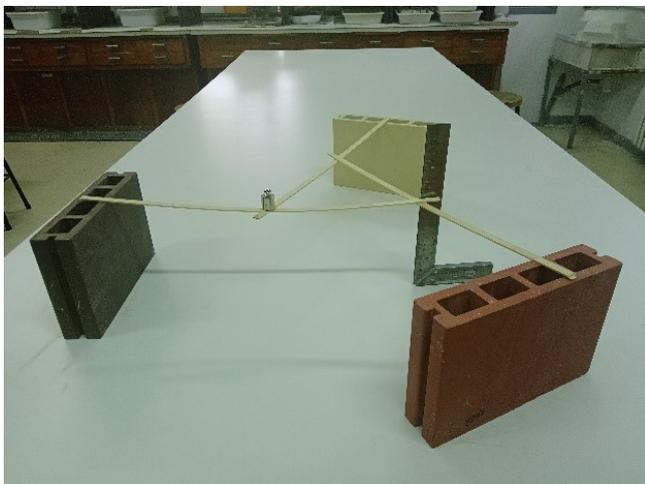
Figure 5. Vertical deflection at the end of member into reciprocal structure.
