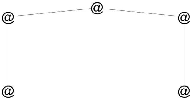
Figure 1. The scheme of the kind of portal frames studied with all joints semi-rigid
