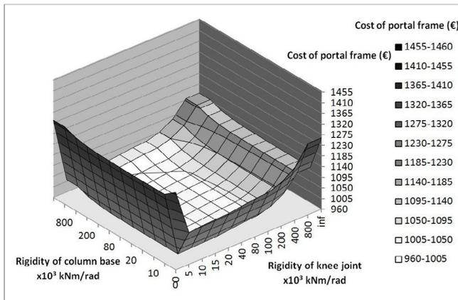
Figure 7. 3D view of the graphic corresponding to 8 m span, 3.5 m column height and 20% slope portal frame at low load level. Rigidity of ridge joint  $80 \cdot 10^3$  kNm/rad
