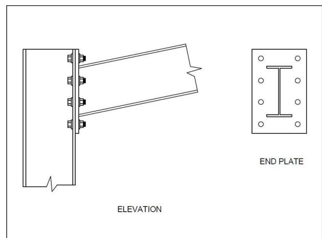
Figure 4. Model of the knee joint considered, when the rigidity value is greater than  $20 \cdot 10^3$  kNm/rad
