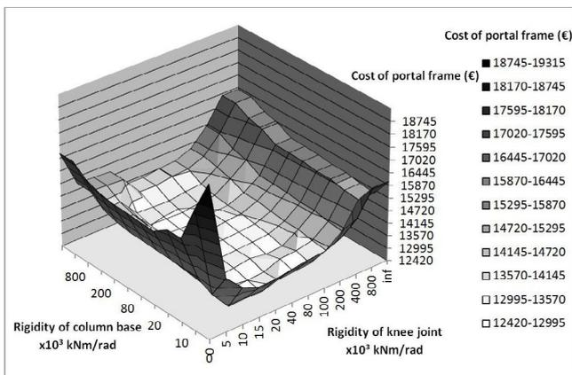
Figure 8. 3D view of the graphic corresponding to 15 m span, 10 m column height and 10% slope portal frame at high load level. Rigidity of ridge joint  $200 \cdot 10^3$  kNm/rad
