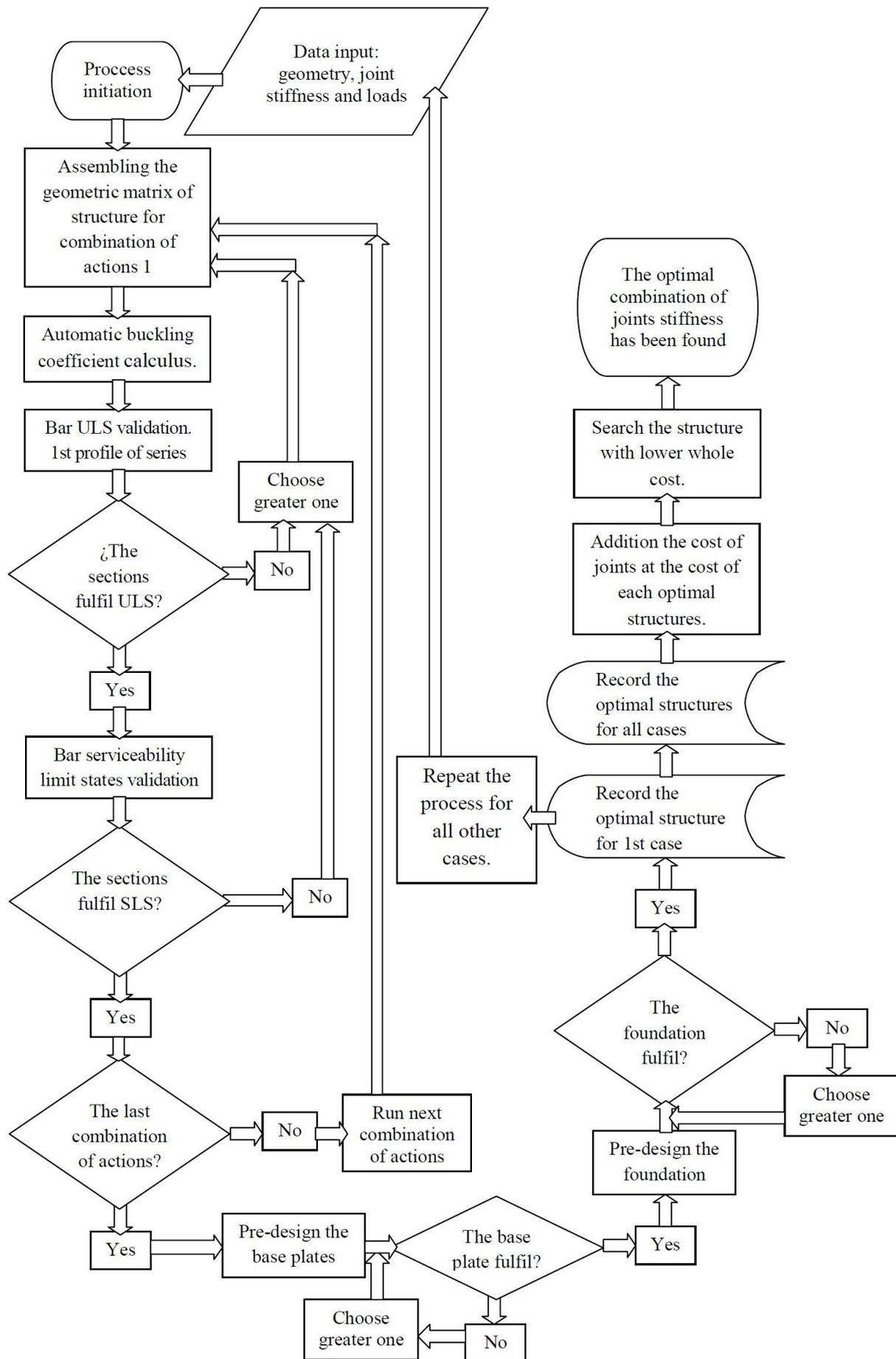
Figure 6. Flow chart of the process of structural design in an optimization context.
