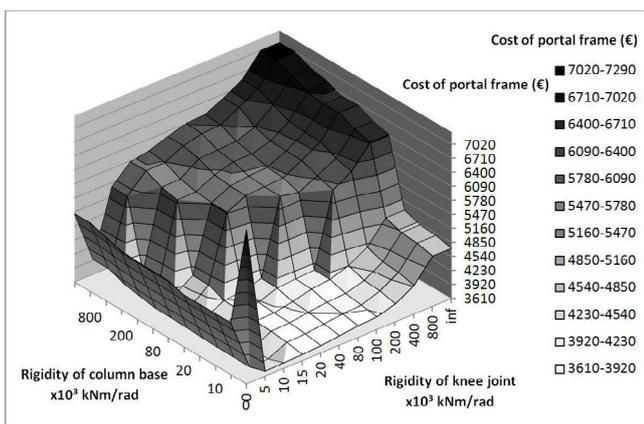
Figure 9. 3D view of the graphic corresponding to 10 m span, 3.5 m column height and 15% slope portal frame at high load level. Rigidity of ridge joint  $10 \cdot 10^3$  kNm/rad
