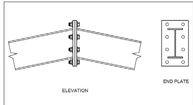
Figure 2. Model of the ridge joint considered for the study
