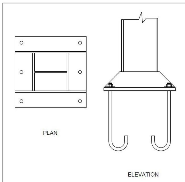
Figure 5. Model of the column base considered
