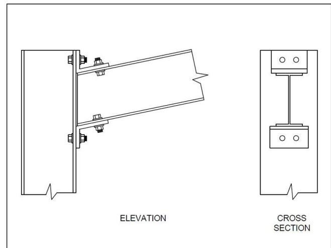
Figure 3. Model of the knee joint considered, when the rigidity value is equal to or less than  $20 \cdot 10^3$  kNm/rad
