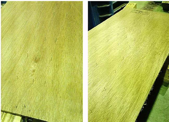
Figure 21. Photograph of the condition of sheathing nails after the three-point bending test of prototype *CP2a\_1t\_c*.
