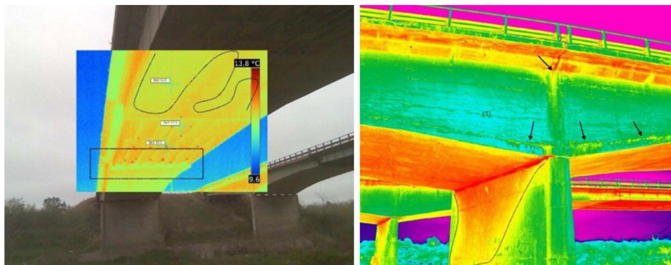
Figure. 5. Infrared (IR) aerial photography showing various deficiencies. Source: Courtesy of Falcon High Tech.
