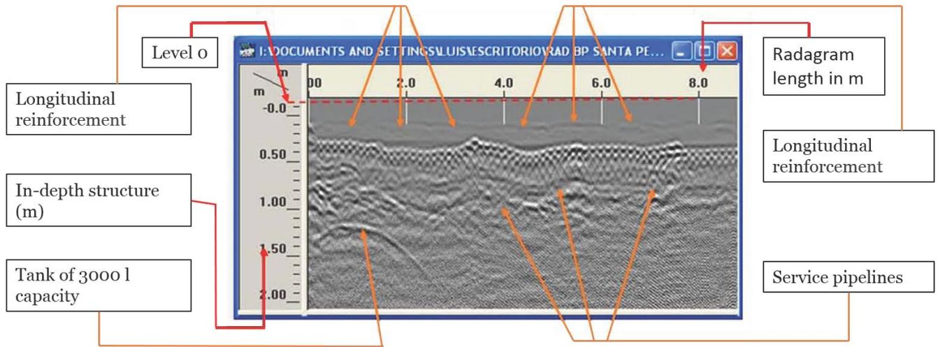
Figure 1. Radargram of a concrete flooring, without processing, as seen by the operator.
