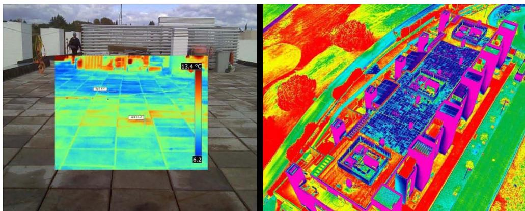
Figure 3. Thermographic surface image and Aerial infrared photography from 60 m. Source: Courtesy of Falcon High Tech.
