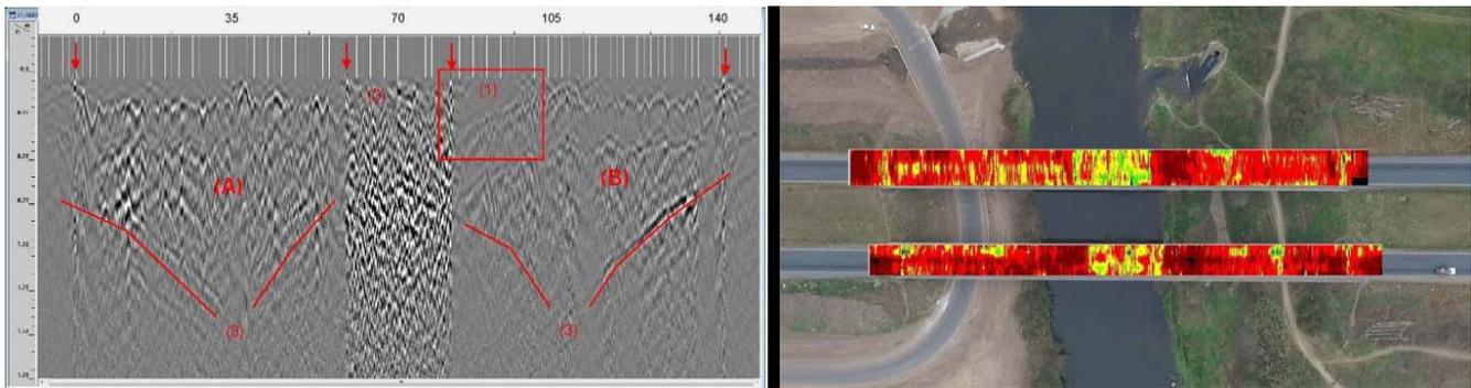
Figure 6. Radargram 202. 1.75 m deep. It shows deficiencies close to the central isostatic zone, and 3D geo-radar of both boards, with detection of the dielectric constant associated with fractures, fissures and discontinuities. Source: Courtesy of Falcon High Tech.
