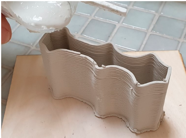
Figure 7. Using 3Dclay part as recyclable mold for cement
